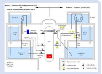
ment geometrical considerations. The GDCS and ADS are the plant's Emergency Core Cooling System (ECCS).
